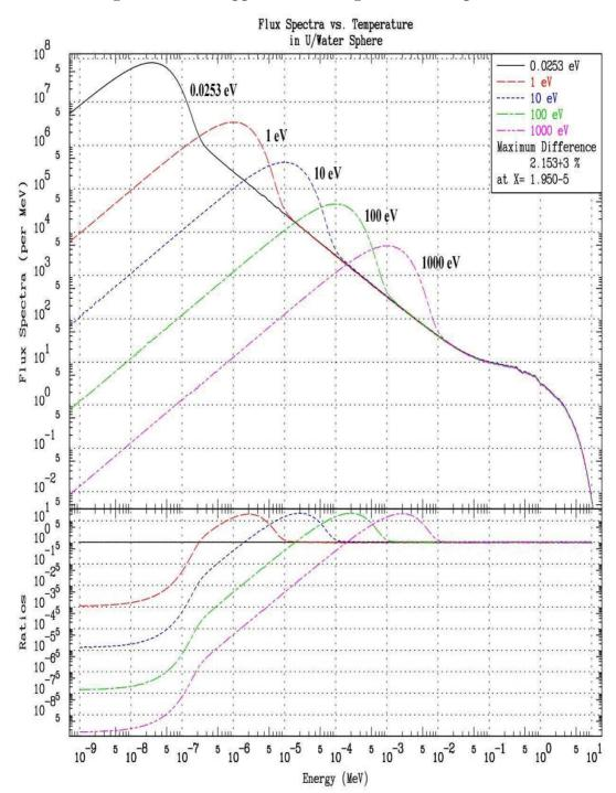
Fig.4: Effect of Doppler Broadening on Neutron Spectrum
