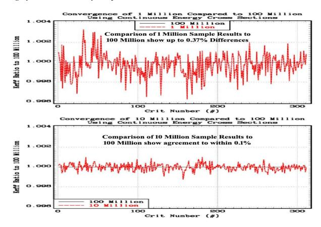
Here to illustrate convergence I used **Continuous** energy cross sections to compare results for 311  $^{235}$ U slow critical assemblies [8] for:  $10^{+6}$ ,  $10^{+7}$ ,  $10^{+8}$ , and neutron samples. The above figures show that  $10^{+6}$  results differ from the  $10^{+8}$  results by up to 0.37%, and  $10^{+7}$  results have converged to within 0.1% of the  $10^{+8}$ .
