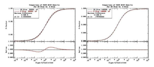
That is not to say that there is anything wrong with the 20 bands and it gives good answers, but for this application 20 bands simply isn't needed; 2 bands are sufficient as long as these 2 band parameters are defined using the multiband definitions to exactly conserve important moments of the flux, as I have done above; AS WITH ANY DISCRETE QUADRATURE, SUCH AS LEGENDRE QUADRATURE USED BY Sn CODES, THAT IS THE KEY.
