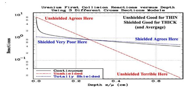
Through Thick or Thin: The above figure demonstrates that in order to reproduce the spatially dependent Total Reactions we need Unshielded group averages for THIN, or small, depths (or thicknesses), and Shielded group averages for THICK, or larger, depths (or thicknesses) to reproduce spatial averages. With only one degree of freedom (the group average) normal multi-group models cannot simultaneously satisfy both extremes.
