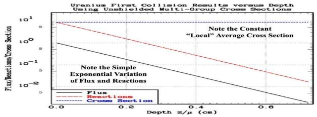
In the above figures the most obvious differences are because using continuous energy cross sections the "local" ( $z/\mu$  dependent) total cross section is variable, whereas with multi-group cross sections, by definition, the total cross section in any one group is a constant.
