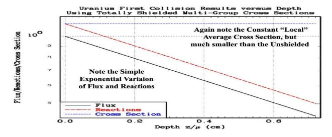
Below when we compare the **total reaction rates vs. depth** for these three cross sections models, we can see that the **Unshielded** model yields the same reaction rate at the surface but varies enormously everywhere else. Whereas **Totally shielding** yields much lower reaction rates near the surface ( $\sim 8$  times lower), but pretty good agreement deeper into the Uranium
