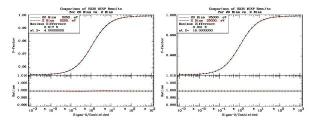
Using 20 or 2 bins, for  $^{238}$ U we see differences up to 0.328% at the lower energy limit (20 keV) and up to 0.005% at the upper energy limit (near 149 keV); there is a small difference at 20 keV and virtually none at 149 keV. There is little significant difference that affects integral results (which help to explain why we saw no significant difference above for the  $K_{eff}$  values).
